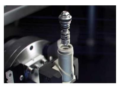
As a world premiere, GF Machining Solutions gives the operator the possibility to work with open or closed guides, thanks to a quick and simple system of interchangeable cartridges on the CUT X series.
