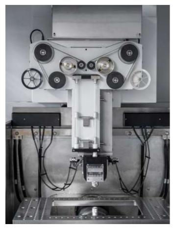
The CUT X machine includes two identical, symmetrical wire circuits for simple, fast roughing and finishing, optimal cutting speed and accuracy and double wire autonomy.
