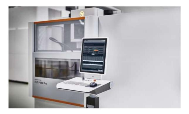
The new human machine interface (HMI) Uniqua, here on the CUT P 550 Pro, offers optimal functionality and ergonomics for every skill level.
