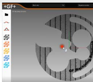
Perlage decoration toolpath, created with LaserCAM™
